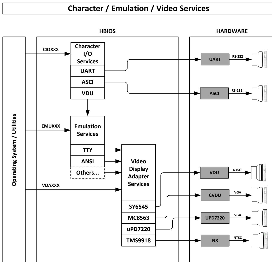
Normally, the operating system will simply utilize the CIOXXX to send and receive character data. The Character I/O Services will route I/O requests to the specified physical device which is most frequently a serial port (such as UART or ASCI). As shown above, if the CRT device is targeted by a CIOXXX function, it
